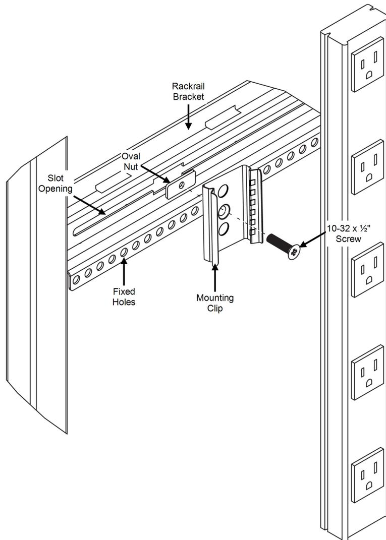
4. Repeat the previous steps to match the hardware amounts (oval nuts, screws, and clips) to the amount of rackrail brackets in your enclosure.
