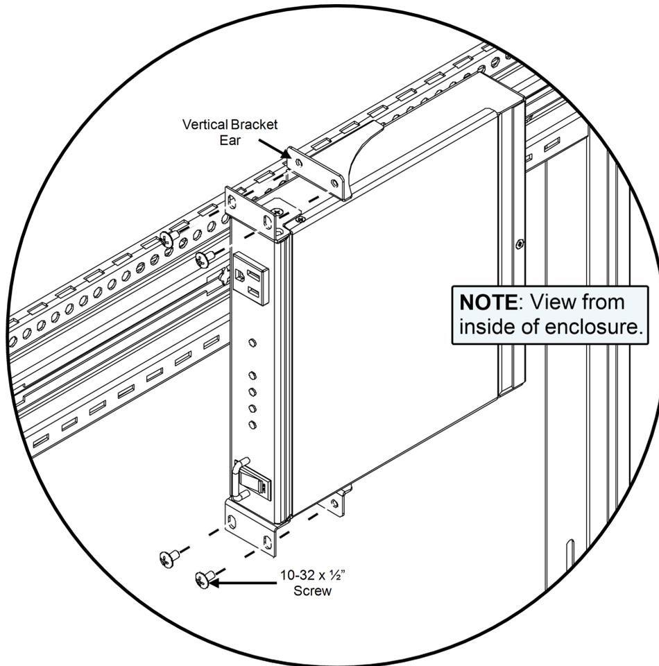
2. Use a #2 Phillips screwdriver and (4x) 10-32 x 3/8" screws through the holes on the ears of your PDU and into the ears on the vertical bracket as shown.
