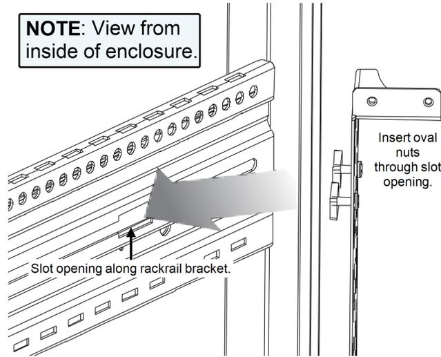
5. Make any final positioning adjustments on the vertical bracket obrounds and the specific location along rackrail bracket, and then use a #2 Phillips screwdriver to fully tighten both screws.
